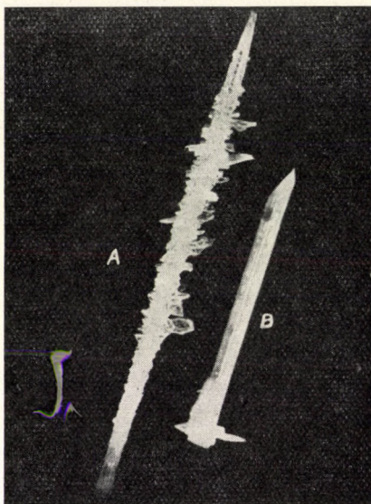
Fig. 4. Rod- and needle-like ZnS dendrites. On crystal B it is well observable that the continuation of the dendrite is a hexagonal, hollow crystal
