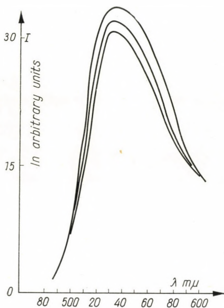
Fig. 7. Spectra of layers, which were treated with 1% soda solution at 80^{\circ}\text{C} , before the adsorption. The different curves belong to the different oxidizing times
