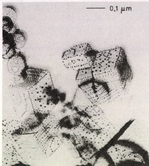
Fig. 6. Evaporation structure: Steps on the whole particle surface
