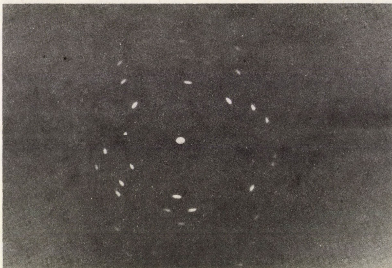
Fig. 4. Laue patterns from slides cut from: a) sample No. 57 (BT), exposition 60 hours; b) sample No. 28 (VPT), exposition 20 hours. The diffraction patterns were obtained in transmission with a TUR-M apparatus W-anode, U = 55 kV, I_a = 12 mA
