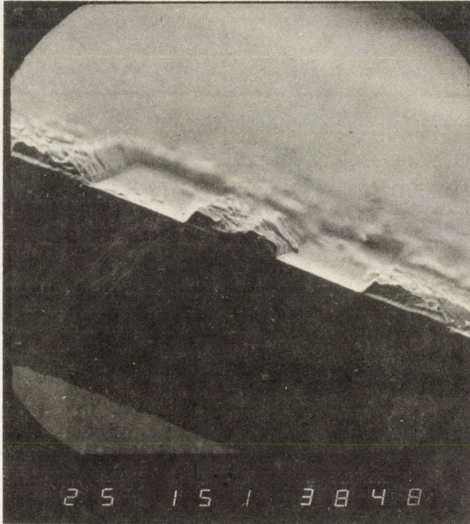
Fig. 4. Cleavage cross section of a AlGaInSb epitaxial layer grown onto polycrystalline GaSb wafer
