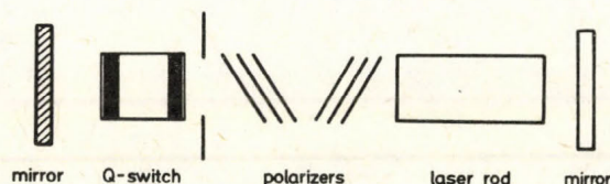
Fig. 1. Nd-glass laser switched by KDP 0^\circ Z cut electrooptic modulator
