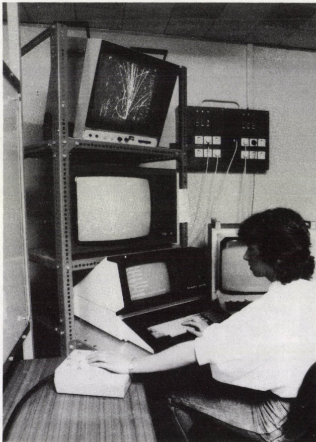
Fig. 3. The monitor and switchboard of the RIMA automatic measuring device for the analysis of the streamer chamber pictures in the Central Research Institute for Physics, Budapest
