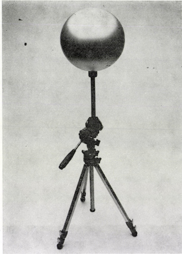
Fig. 3. Low level chamber on tripod.
