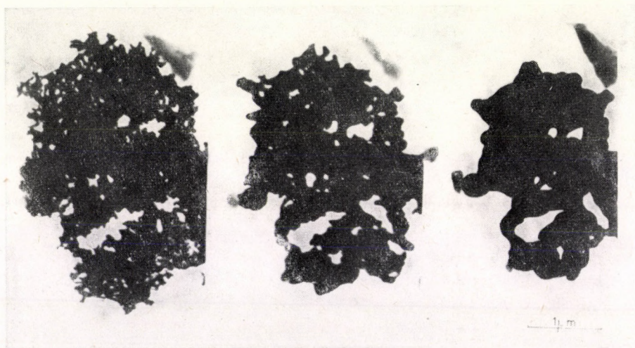
Fig. 3. Gradual sintering of the crystals of platinum black containing Si during a heat treatment at 1200 K
