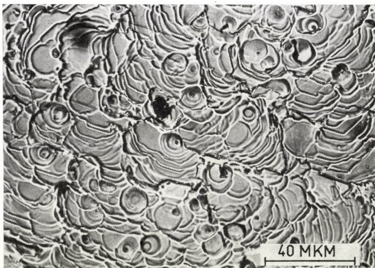
Fig. 3. Typical shape of surface of thick diataxial layer observed using interferential contrast
