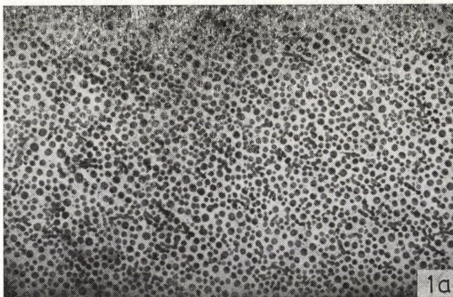
Plate (1a). 9000 times magnified photograph of Te film 0.05 \mu\text{m} thick deposited on cold mica substrate
