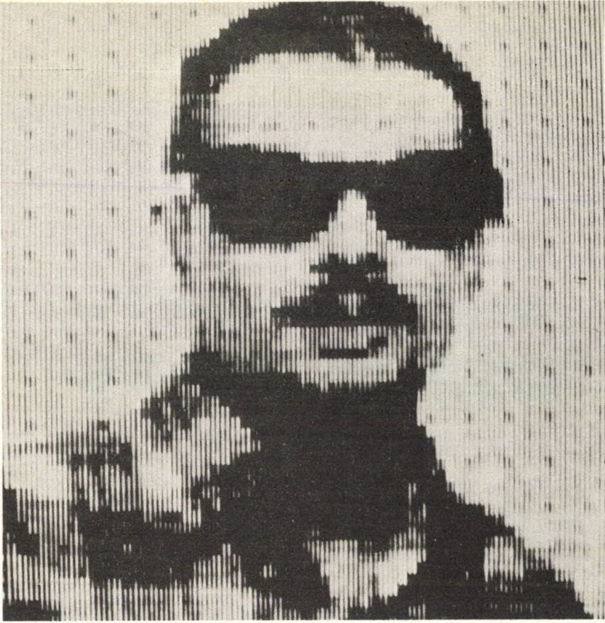
(b) Compression ratio 4:1, S=200 , p=8 , zonal filtering (8a), quantization (10b), nonadaptive algorithm.
