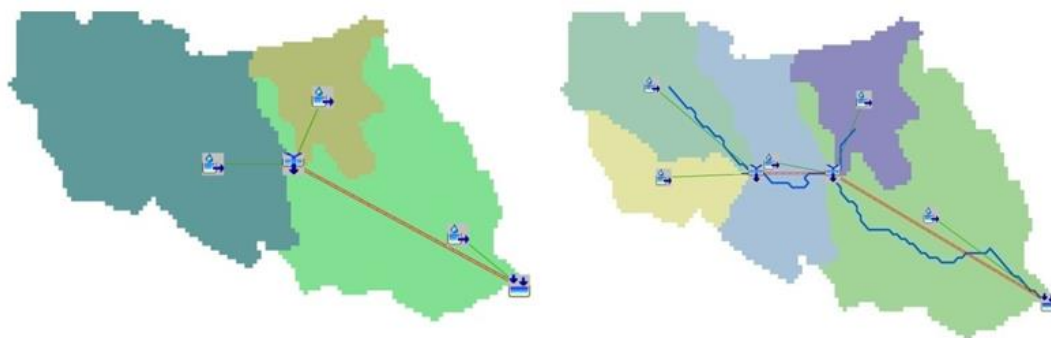
Figure 5. Basin model of Bükkös watershed with three (left) and with five (right) sub-basins in the lumped model
