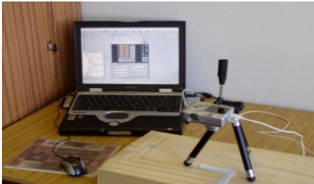
Figure 8. Apparatus for measuring the kerf width
