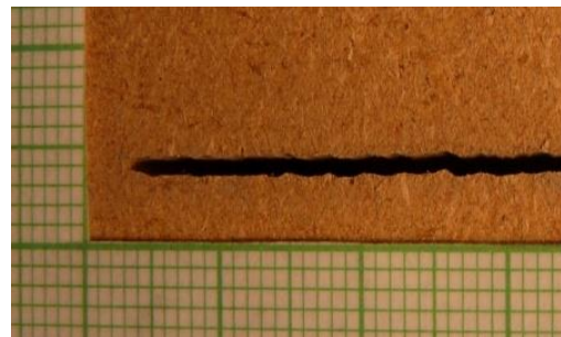
Figure 9. Digital picture of kerf on the MDF verification sample, kerf on the entry side of the material (left) and kerf on the exit side of the material (right)
