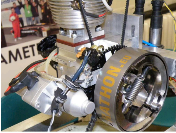
Figure 6: Setup for measuring the instantaneous torque
