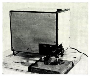
Fig. 1. Equipment for testing of surface roughness and wear resistance of flooring
