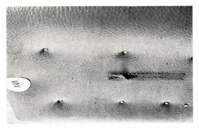
Fig. 5. Surface of Dynafarm floor after mechanical rubbing (friction) for two minutes
