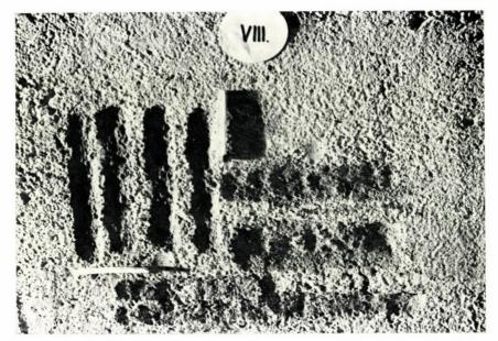
Fig. 4. Surface of Graboplast floor after mechanical rubbing (friction) for two minutes
