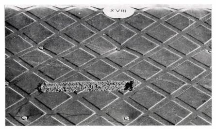
Fig. 6. Rubber floor (pyramid pattern) after mechanical rubbing (friction) for five minutes
