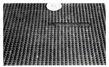
Fig. 7. Surface of asphalt "x" floor after mechanical rubbing (friction) for five minutes
