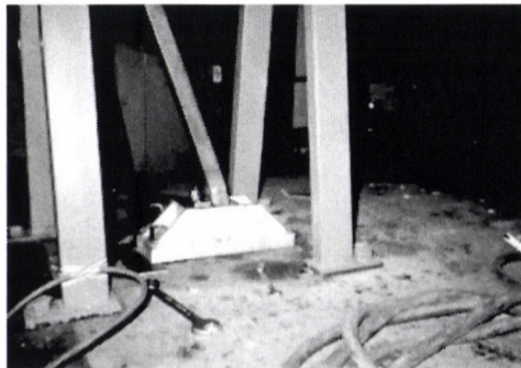
Fig. 13. The basis of the specimen, permanently yielded and buckled after the experiment
