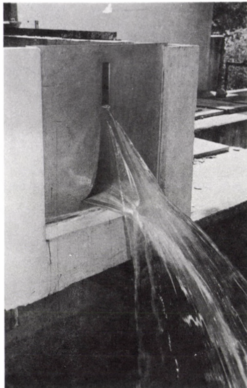
Fig. 6. Side view of flow through modified Rankine half body weir, showing nappe
