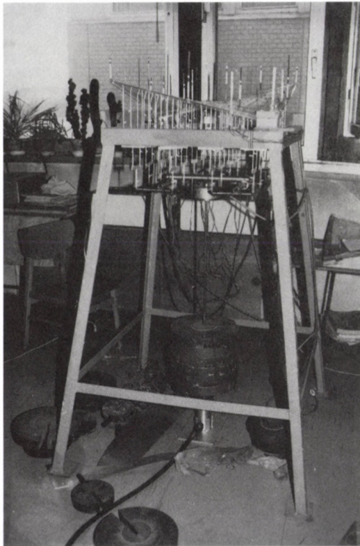
Fig. 7b. Load transfer to the rocker system (Models 1, 2, 3, 6)
