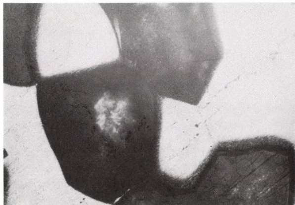
Fig. 5. Grain structure of ground and polished but not etched soft aluminium wire Magnification: 100x
