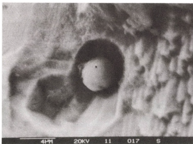
Fig. 3. Magnification: 5000 x Chemical composition of steel, %: C - 0.11; Mn - 1.45; Si - 0.41; S - 0.008; Al - 0.018; V - 0.06; O - 70 ppm Chemical composition of inclusion, %: Mn - 51; S - 48.5; V - 0.5
