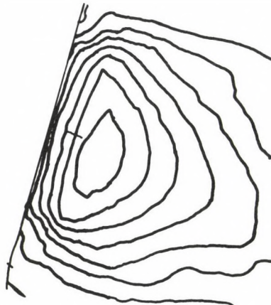
Fig. 5. State of stress in meshing teeth a) according to optical stress analysis /16/; b) reduced stresses according to von Mises; c) reduced stresses below the contact region according to von Mises
