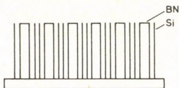
Fig. 6. BN plate—Si wafer arrangement
