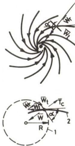
Fig. 9. Flow lines of the vortex sink, and motion of the coal dust particle in a turbulent flow: 1 - vortex line, 2 - flow line of the vortex sink
