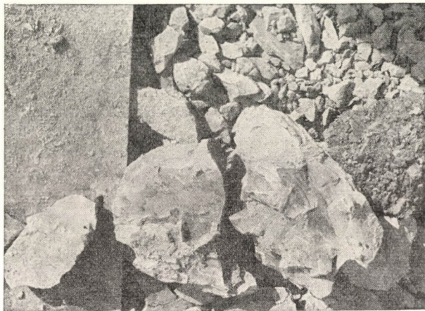
Fig. 4. Fissured clay marl blocks after excavation
