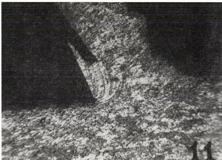
Fig. 13. Chip root micro-section of aluminium alloy Feed e = 0,3 mm rev; cut depth f = 3 mm; cutting speed v = 45 m/min; magnification 63 \times
