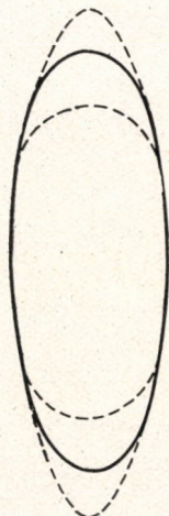
Fig. 2. The part of the arc of ellipse around the small axis does not determine the great axis
