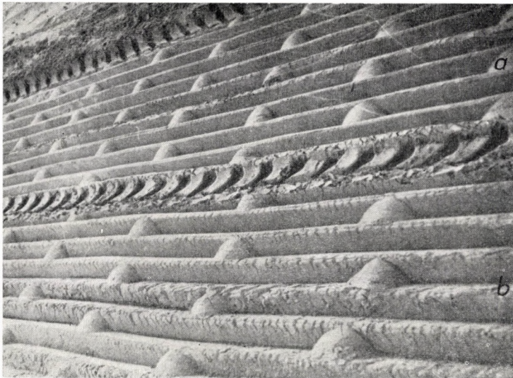
Fig. 12. Working effect of burrow-free ring-roller with various tractive speed values a) — v = 7 km/h; b) — v = 13,5 km/h
