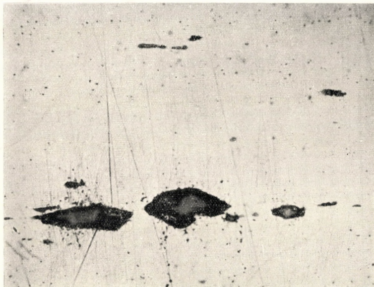
Fig. 7. K_21 test-piece longitudinal section. Aligned rows of SnO 2 in cavities. M = 750 \times
