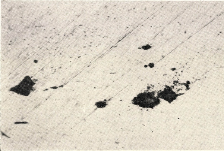
Fig. 10. K 2 - test-piece longitudinal section. The inclusions scattered. M = 750 x
