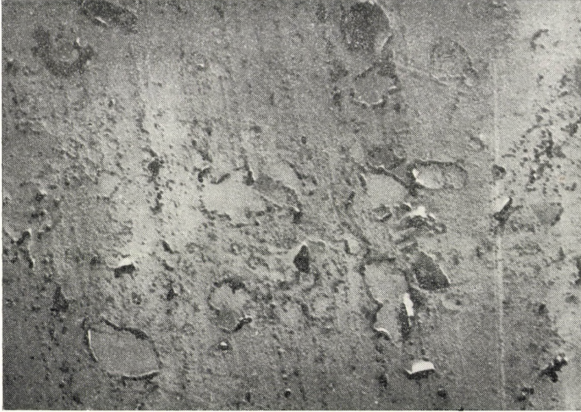
Fig. 2. Surface of gold specimen attacked for 5 sec (16 600 \times )
