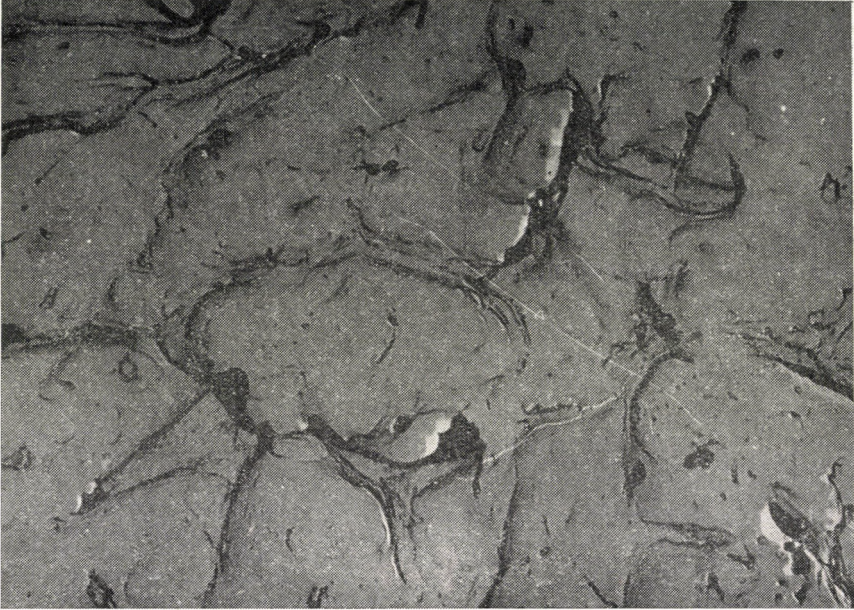
Fig. 10. Surface of a bronze specimen, attacked for 8 sec (12 600 \times )
