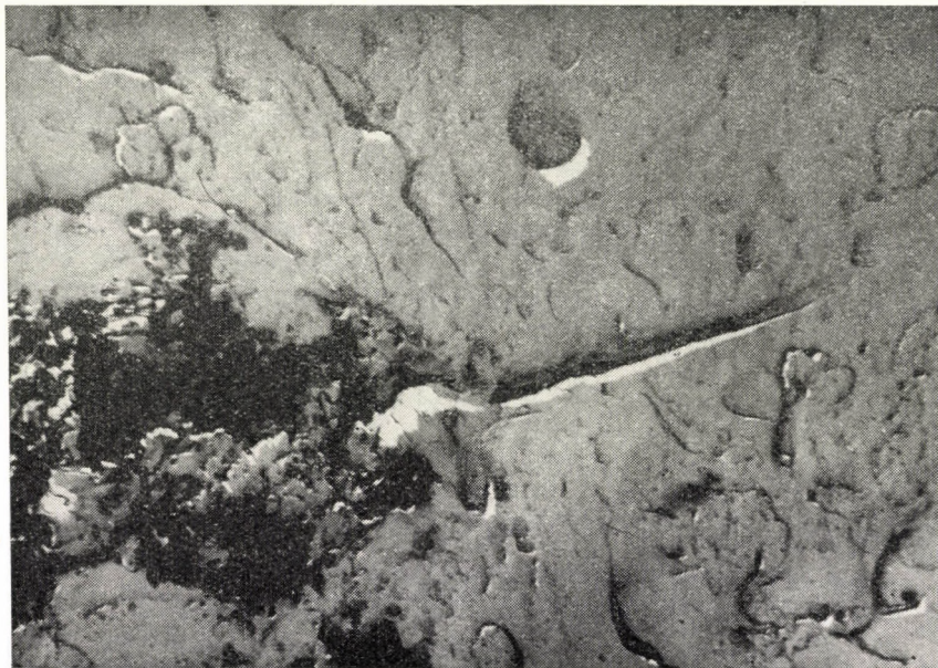
Fig. 6. Surface of aluminium specimen attacked for 5 sec (11 300 \times )
