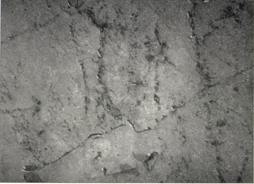
Fig. 4. Surface of a gold specimen attacked for 5 sec, after elimination of a 0,02 mm surface layer (8000 \times )
