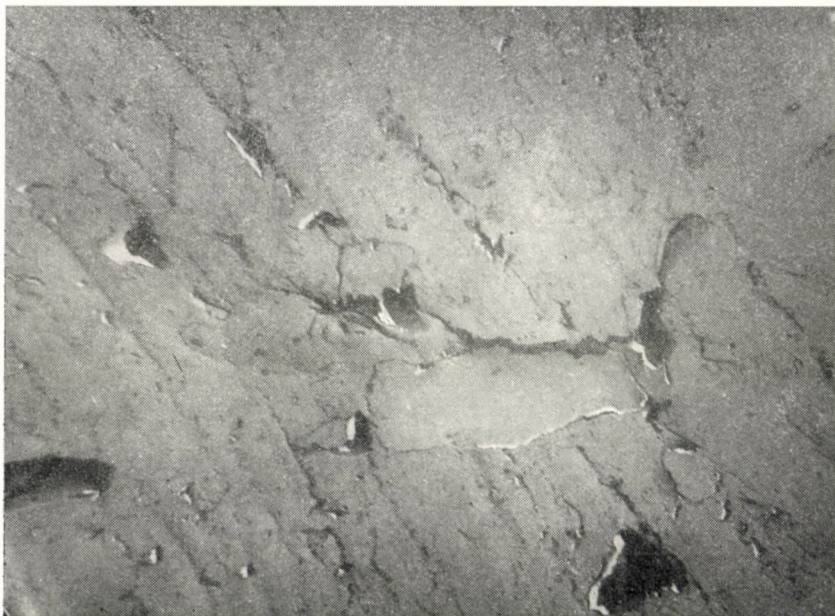
Fig. 8. Surface of a copper specimen attacked for 5 sec (4700 \times )
