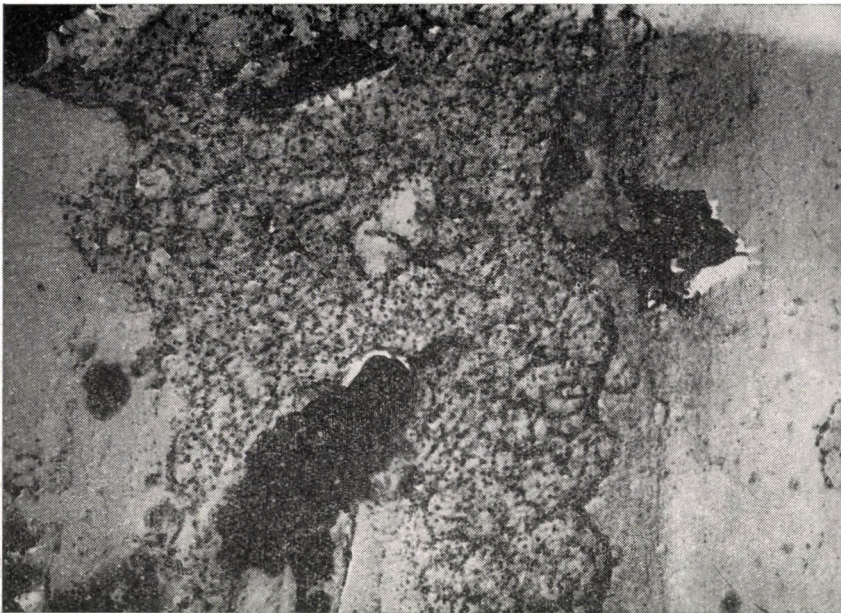
Fig. 17. Surface of carbon steel A 60.11 attacked for 6 sec (14 400 \times )
