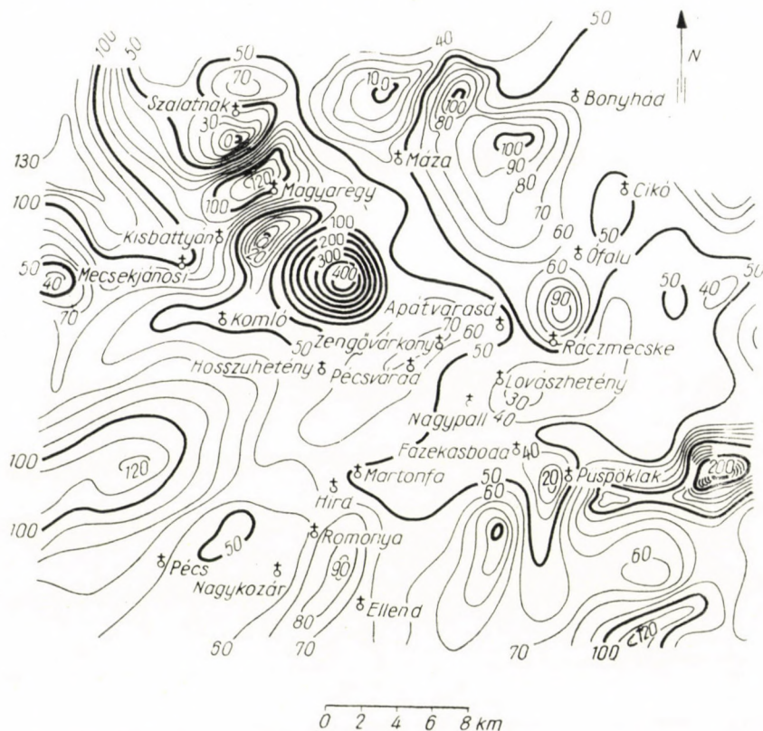
Fig. 7. The anomalies of the vertical magnetic intensity in the Eastern Mecsek (after SCHEFFER)
