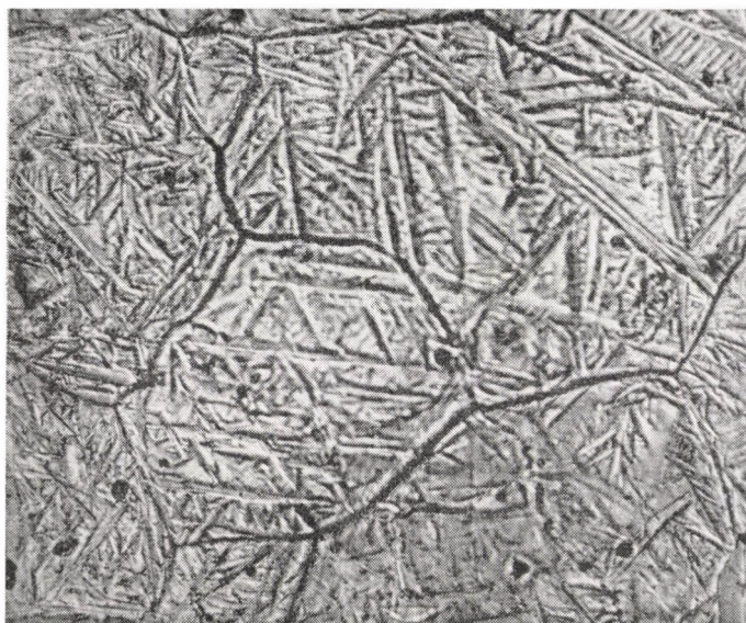
Fig. 9. Ball-bearing steel austenitised at 1150° C for two hours. Slight Nital etch after quenching. 540×
