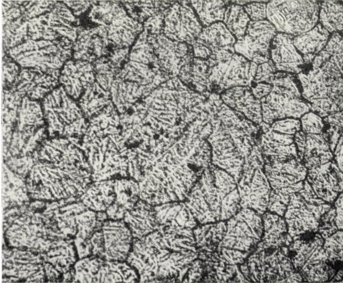
Fig. 4. The sample of Fig. 2 but focused to show the martensitic structure
