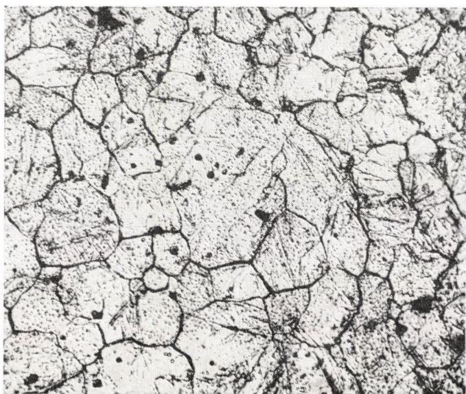
Fig. 2. The same as in Fig. 1 but austenitised at 1050°C for an hour. Grain size ASTM No. 5. Unetched. 180 ×
