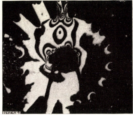
Fig. 5. Pattern of the stress state of feathered gear with top tooth loaded (Pressure on tooth from left to right) [1]
