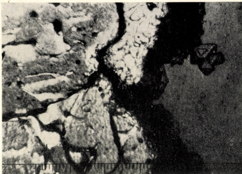
Fig. 5. Cast corundum tank block, in contact with glass containing FeO, MgO. On the right, a layer of spinel and three separate spinel octahedrons. Enlargement: 150 \times 1 \text{ sc.} = 10 \mu . P. light
