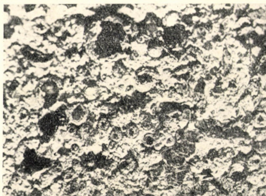
Fig. 6. Spherical shells of graphite at the surface of a cast bar of hypereutectic composition and molten in vacuum
