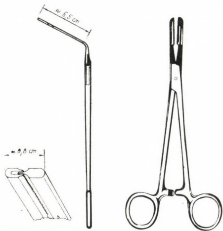
FIG. 7. The intestinal clamp used by us grasps the affected portion of the intestinal wall only over a very narrow surface and thus electrocoagulation is easy to perform. The densely serrated jaws ensure perfect closure and fixation of the intestinal stumps
