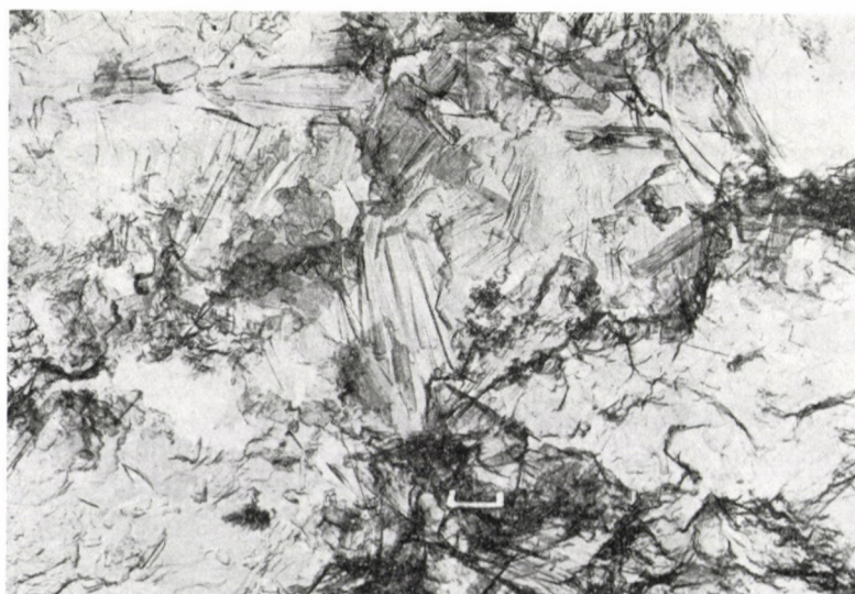
Fig. 3. Transmission electron micrograph of the block formation of mordenite in the volcanic tuff. Magnification: \times 10,000
