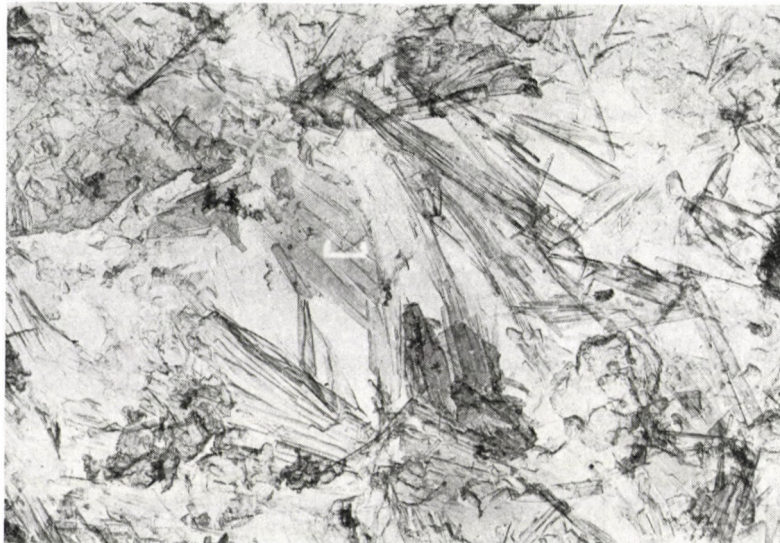
Fig. 2. Transmission electron micrograph of the replica prepared from a fracture surface of the rock. Needle-like individual crystals of mordenite. Magnification: \times 10,000
