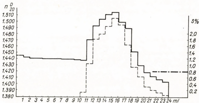
Fig. 5. Gas oil from Nagylengyel 20 ml; silica gel ( 105 \mu ), 50 ml; butanol, 40 ml; small column 3 hrs.
