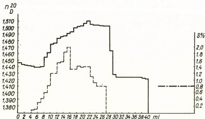
Fig. 6. Gas oil from Nagylengyel 20 ml; silica gel ( 105 \mu ) 50 ml; methanol 20 ml + benzene 20 ml; small column 3 hrs.
