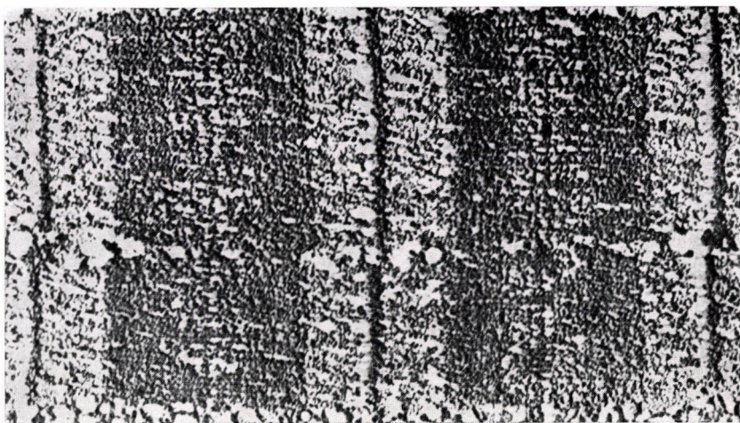
Fig. 5b. The contrasting of the section is the same as that in Fig. 5a, but the direction of steaming is parallel to the direction of the fibrils. The longitudinal structure can hardly be recognized, but there appears a well recognizable transversal structure ( \times 30\,000 )
