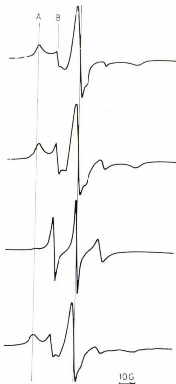
Fig. 1. Epr spectra of spin labelled glycerinated muscle fibers (label II). The uppermost curve shows the epr spectrum of the preparation before treatment, the second spectrum was taken after heat denaturation, the third curve shows the epr spectrum after urea-induced denaturation. At the bottom the epr spectrum of the spin labelled fibers is presented after the experimental procedure. The epr spectra were not normalized to the central line
