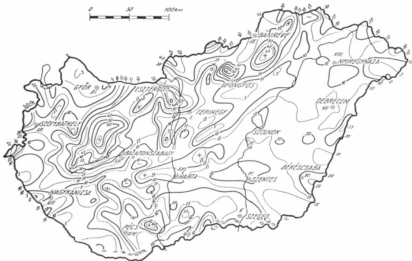
Fig. 2. Representation of the free air gravity anomalies computed from point gravity values using the Int. Gravity Formula (1930) and the Potsdam gravity system. The contour interval is 5 mgal (after Renner 1959)
