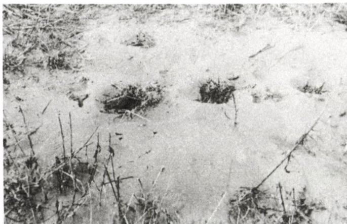
Fig. 15. Sand geysers in Taksony after the earthquake
