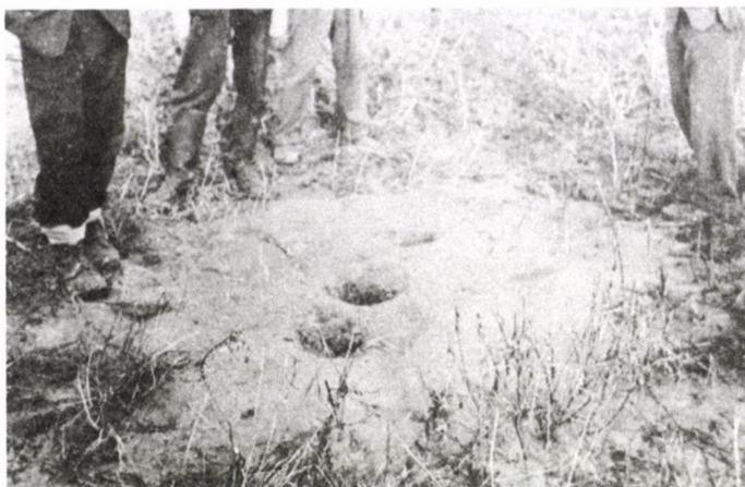
Fig. 14. Sand geysers in Taksony after the earthquake
