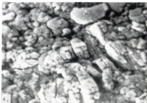
4. Microgranular kaolinite. × 10 000
