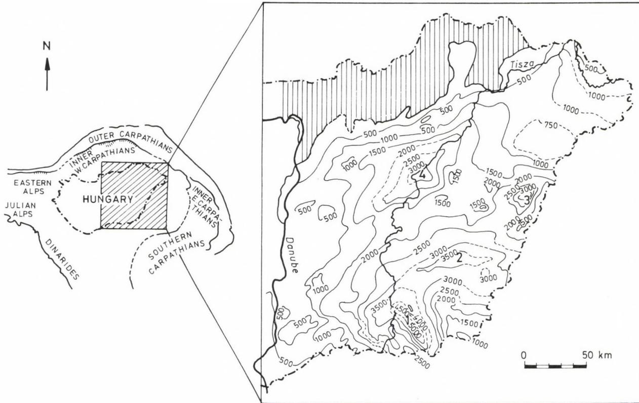
Fig. 1. Location and structural map of the Pannonian (s. l.) basement (after A. Jámor et al., MÁFI, 1986)
