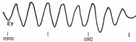
Fig. 1. Example of Pc 3 pulsations in the electric field (period about 23 s)
