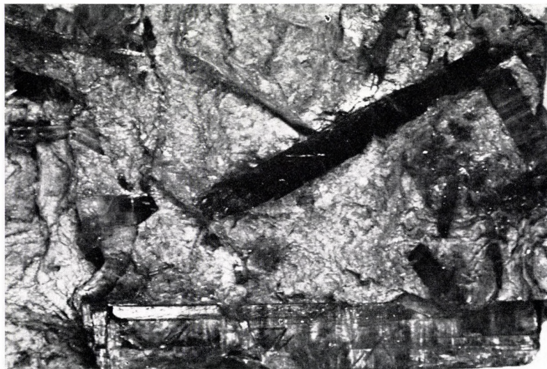
Fig. 4. Kyanite columns and staurolite from the mica gneiss of the borhole Téseny-1, from 156.2 m
