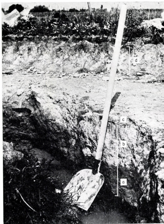
Fig. 5. The carbonate and carbonate mud excavation of Csolyospálos. a ) Red-spotted sandy carbonate rock of looser structure; b ) Hard light-grey carbonate rock; c ) Dark-grey hard carbonate rock; d ) Light grey carbonate mud with meadow soil in its upper part
