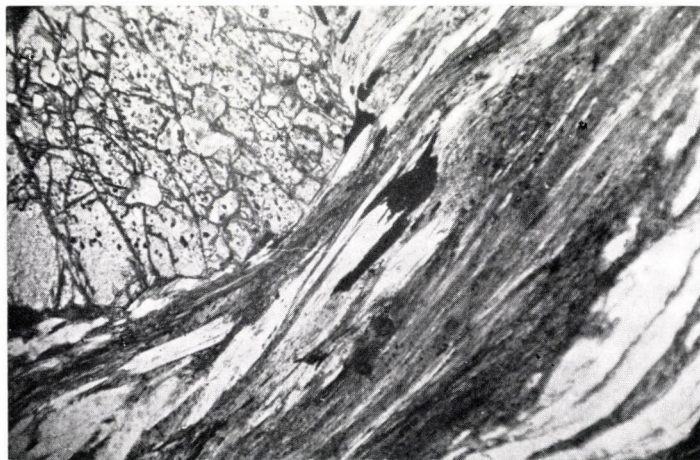
Fig. 3. Muscovite-biotite schist; borehole of Kisdér-1. from 131.6 m; +N, M = 150 ×
