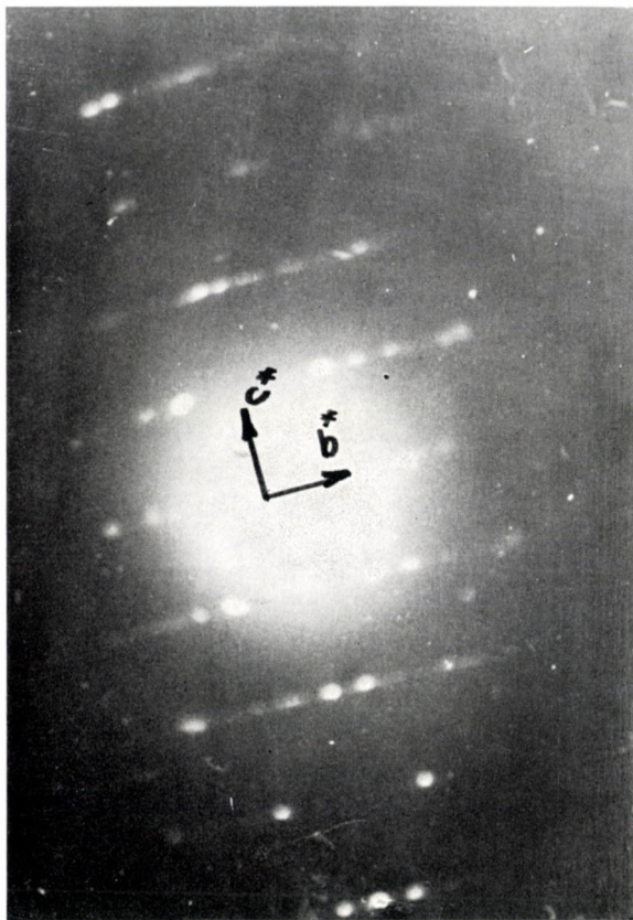
Fig. 3. Selected area electron diffraction pattern of Type II.
