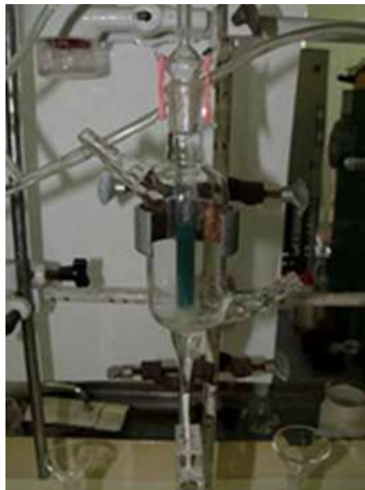
Figure 2. The laboratory ion exchange column
