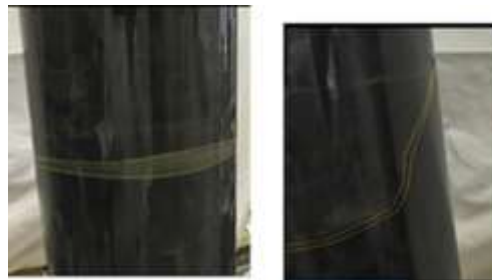
Figure 8. Channelling during high flow rate
