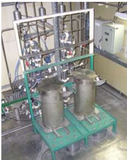
Figure 4. The 12L sorbent columns in lead shield
