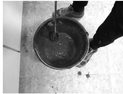
Figure 4 Fresh cement slurry after mixing
