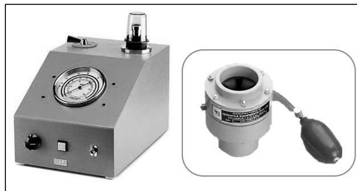
Figure 4 The DISA type permeability measuring device and accessory for sand cores measuring
