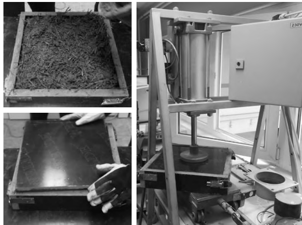
Figure 4 The process of pressing a reed panel
