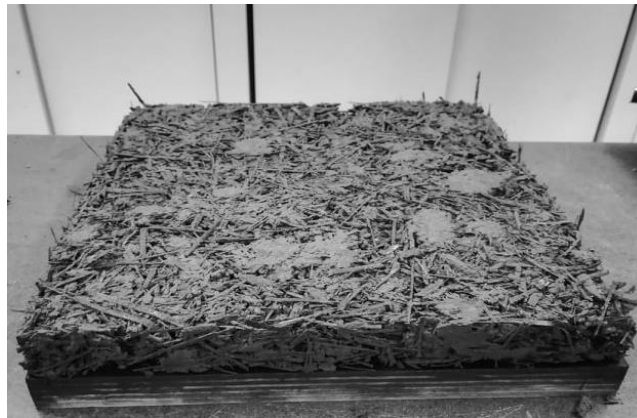
Figure 6 Thermal insulation reed panel
