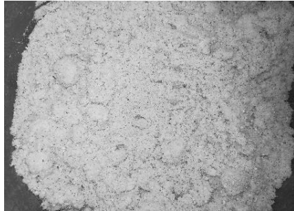
Figure 1 Expanded perlite mixed with water
