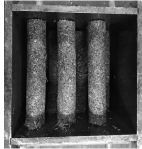
Figure 3 The reed seeds in the mould
