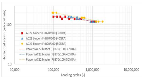
Figure 3. Fatigue curves of AC22 binder (F) asphalt mix manufactured with plain binder and various RAP contents
