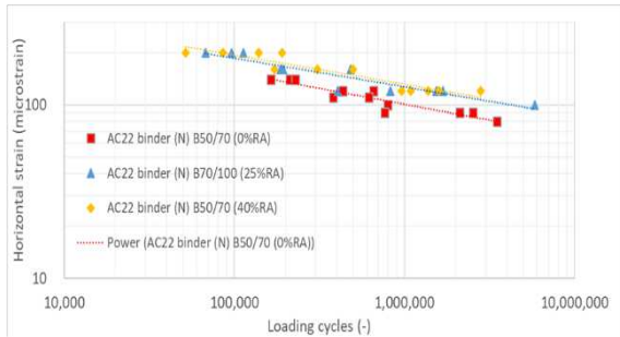
Figure 2. Fatigue curves of AC22 binder (N) asphalt mix manufactured with plain binder and various RAP contents
