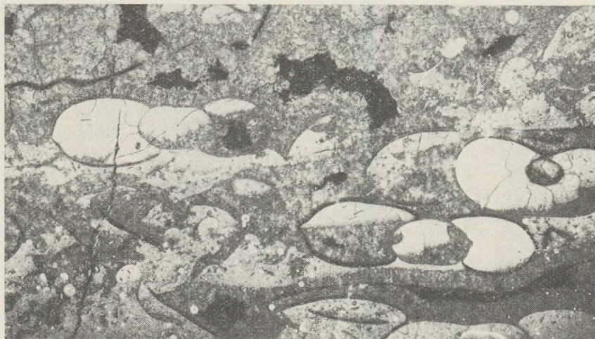
Fig. 6. The middle white limestone (Bed 22). Small ammonites filled up by fine calcareous silt (bottom) and by calcite (top) (magnification: 6.5 x)
