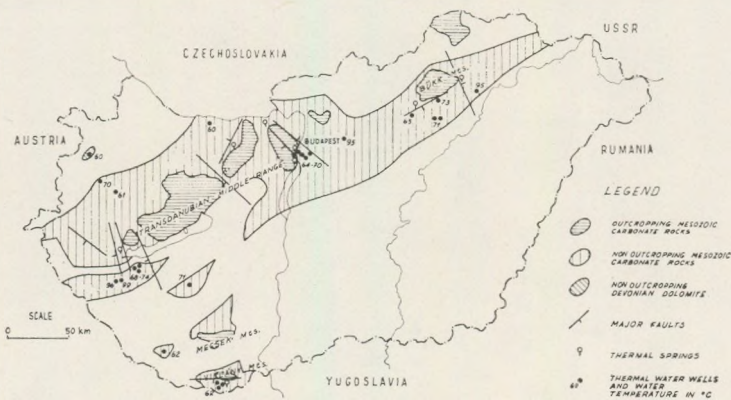
Fig. 11. Thermal water wells and springs issuing from the fractured basements in Hungary. After Korim, 1972.
