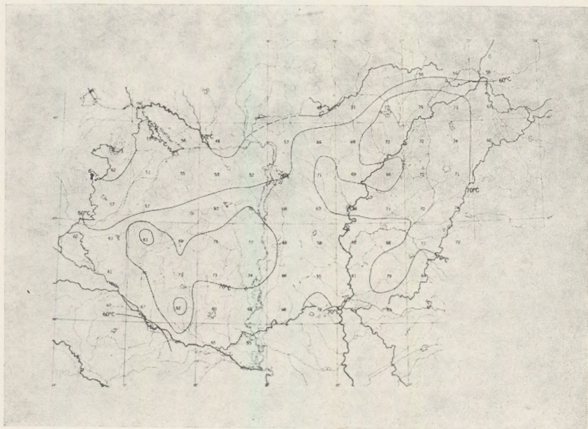
Fig. 2. Mean geothermic temperatures and geoisotherms on the area of Hungary at a depth of 1.0 km
