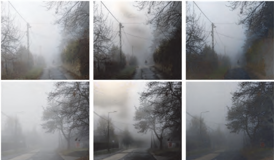
Fig. 5. From left to right: hazy image, dark channel prior, neural network model.
