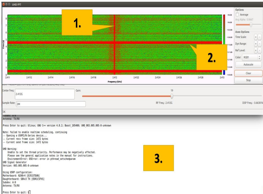
Figure 3: DJI Phantom 2 vision control channel (1) with a pulsed jammer signal (2) generated with uhd_siggen script
