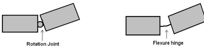
*Figure 2:* Classical coupling (a), Flexure hinges (b).
