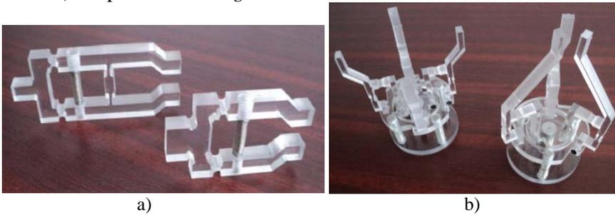
*Figure 8:* Compliant grippers: a) Normal and reverse actuating grippers
