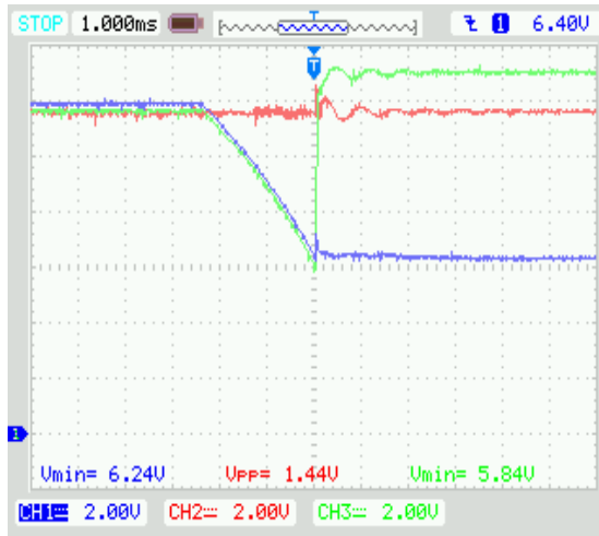
Figure 17: The line transient effect on 1ms time base.
