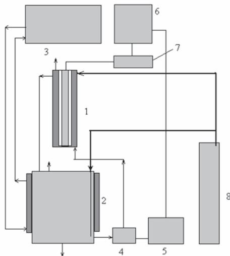
**Figure 1: Schematic diagram of the experimental photoreactor system 1 – Plug-flow photoreactor (PFR); 2 – Buffer vessel; 3 – Ultra-thermostat; 4 – Adjustable flow pump; 5 – Controller; 6 – Power switch unit; 7 – UV source power control unit; 8 – CO<sub>2</sub> cylinder**
