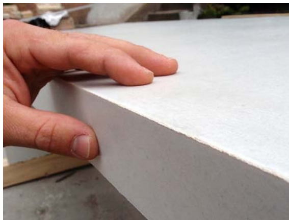
Photo 6: A UHPC bench's edge after being put in formwork, before being chamfered.
