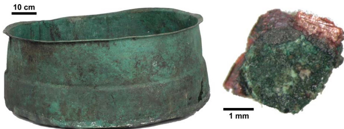
Fig. 6.: Late Roman copper cauldron (photo: A. Dabasi, Hungarian National Museum) and one of the corroded metal samples taken from the cauldron.
